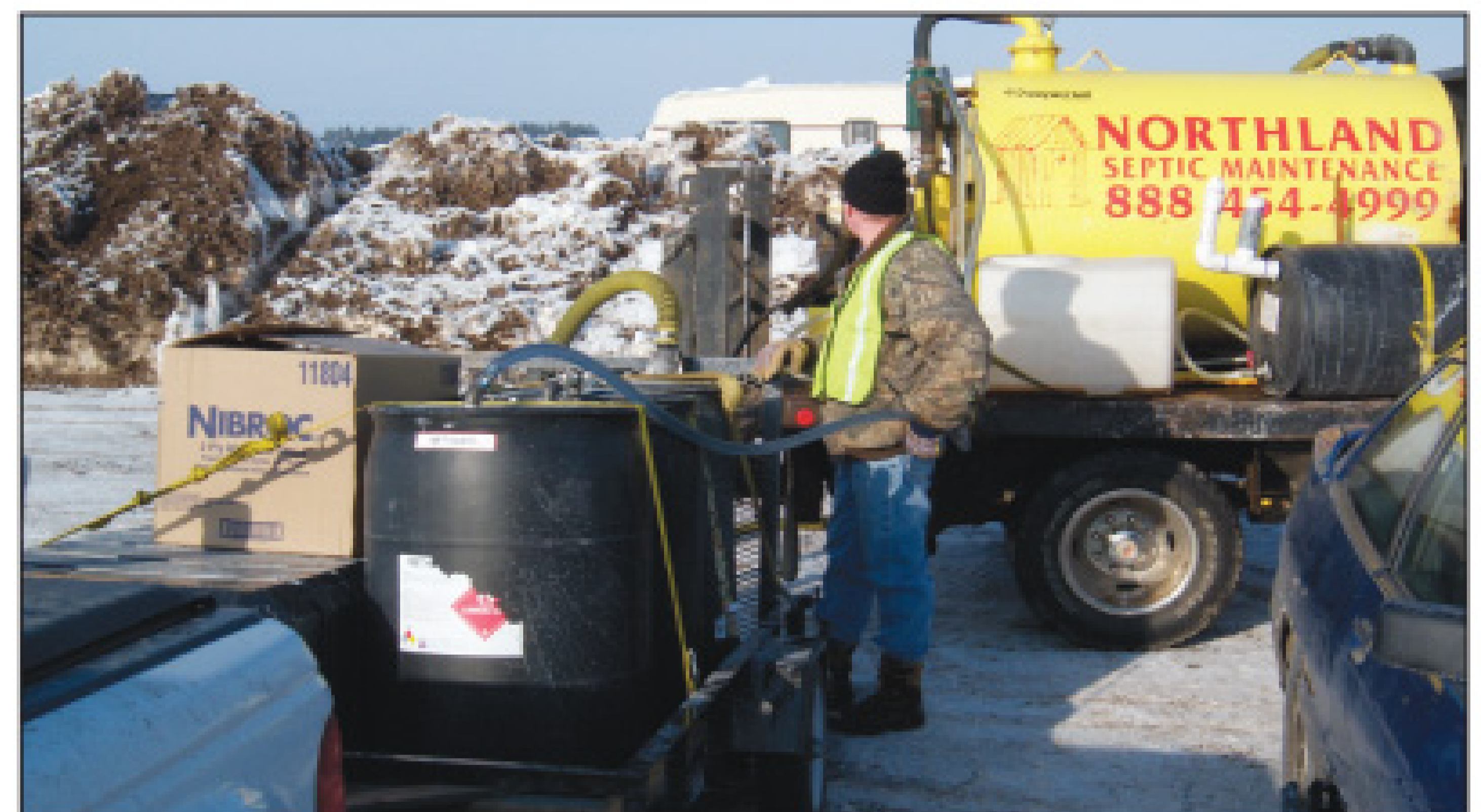
Rick Smith oversees the loading of a portable sanitation truck with water used to recharge units out on winter service.
