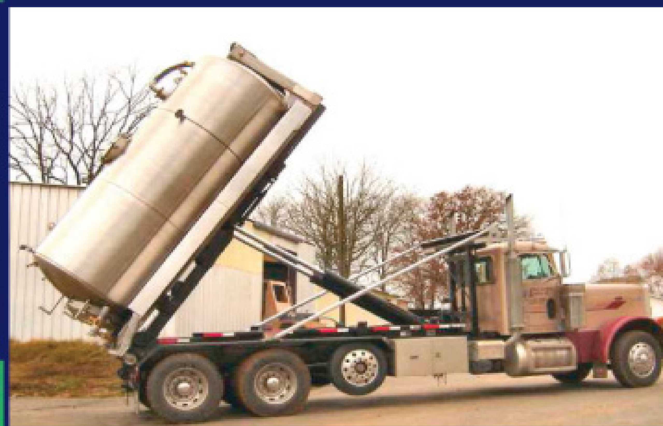
3,200 gallon - All Waste Stainless Steel ROLL OFF TANK
