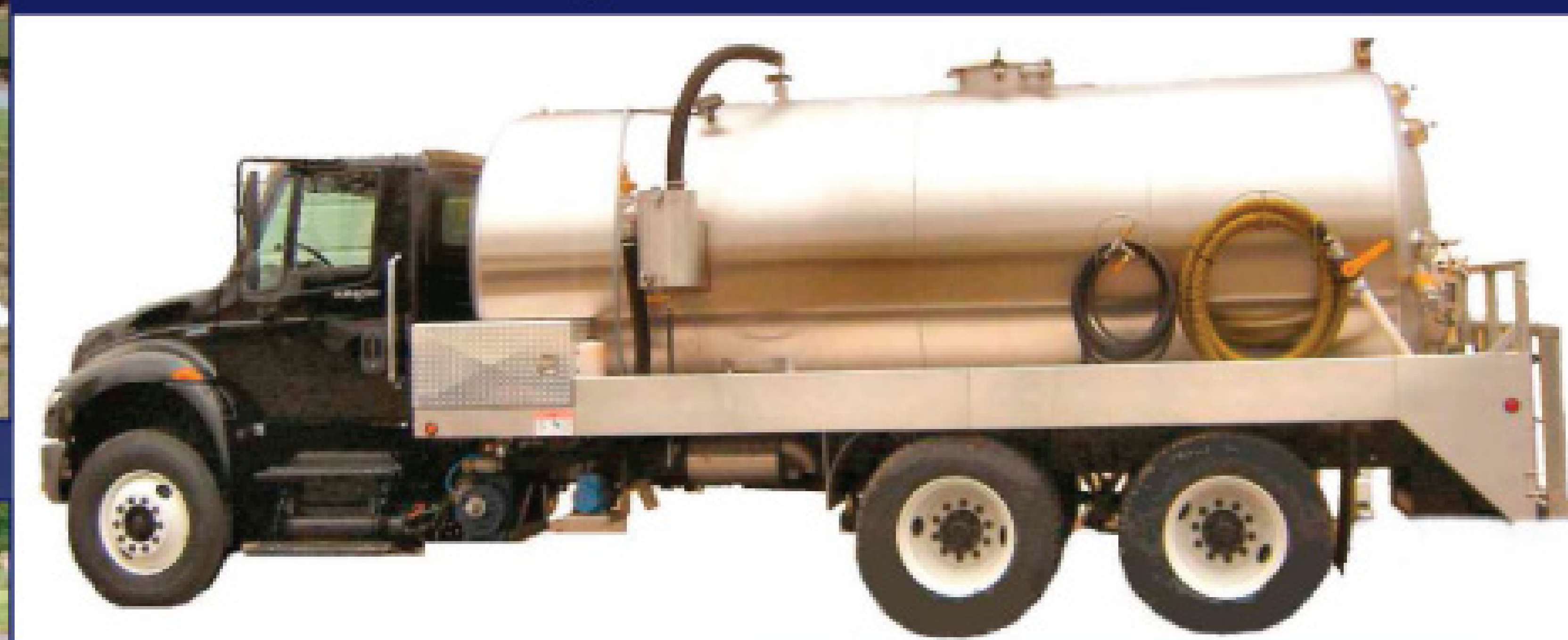
3,600 gallon Stainless Steel tank on a 2008 International Truck. 3,000 Waste - 600 Fresh Water
