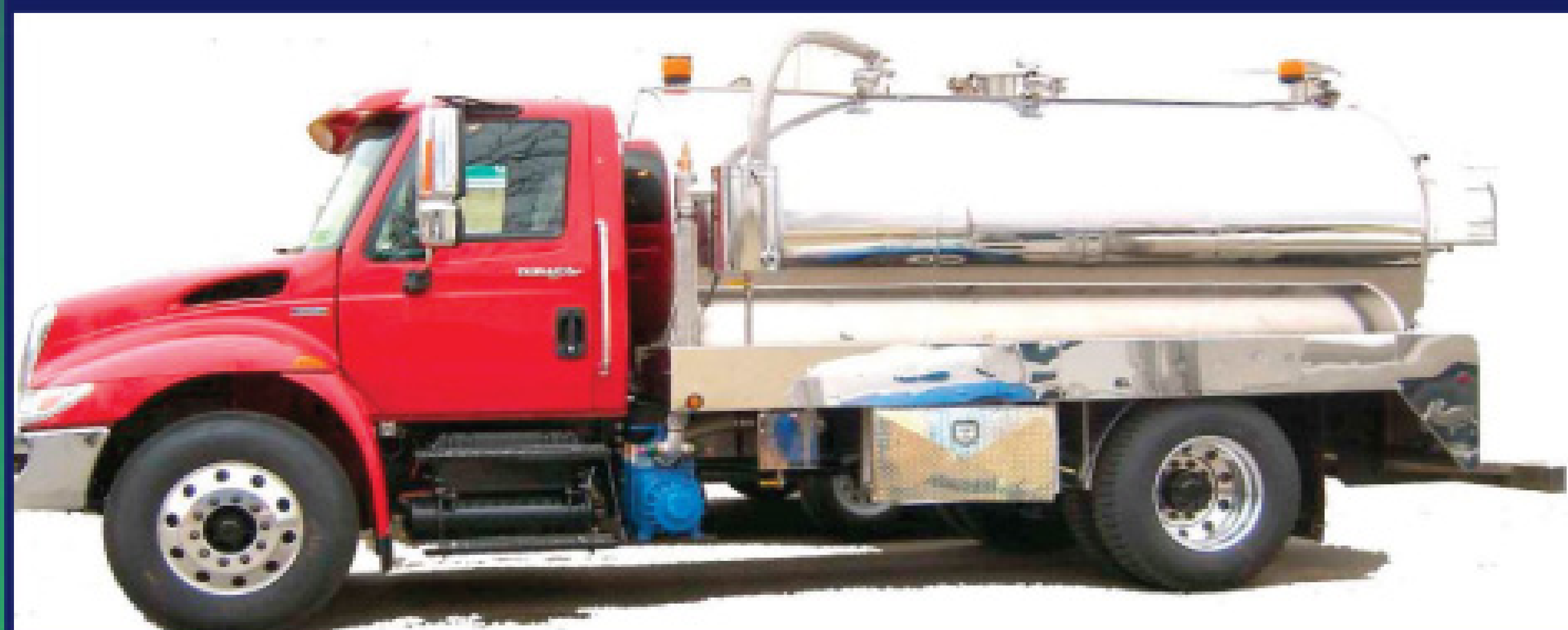
2008 Kenworth T300 with a 1500 gallon Stainless Steel Tank and customized accessories.
