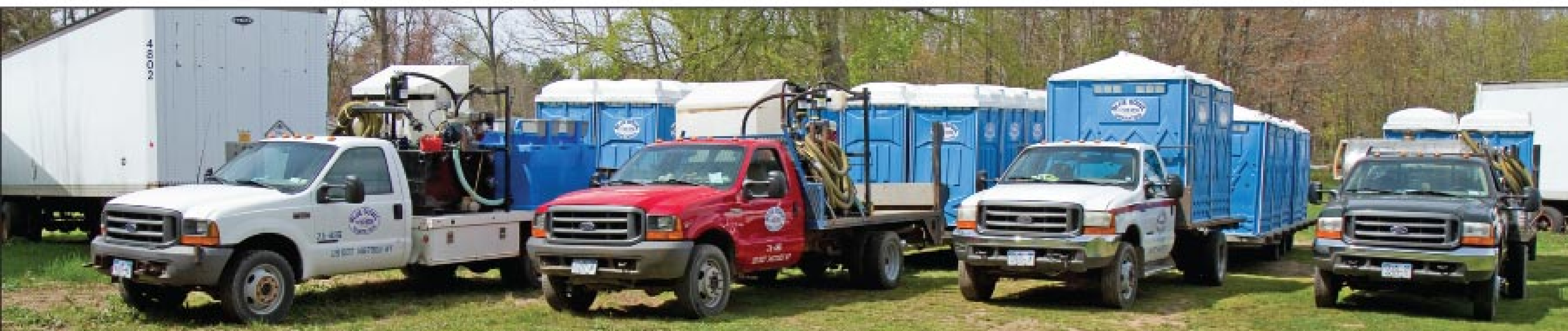
Part of the Blue Bowl Sanitation fleet is ready to roll. The company employs both vacuum trucks with a fixed tank and flatbed trucks with slide-in units to serve a two-thirds special events, one-third construction customer mix.
