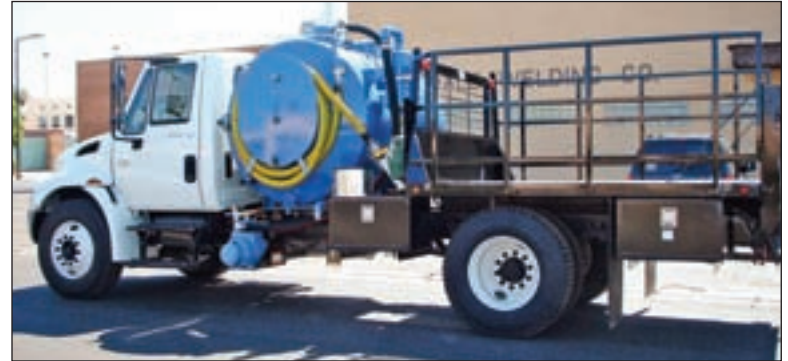
Placing the tank perpendicular to the truck frame and building the freshwater tank into a cylinder at the center of the waste tank is one way to promote even weight distribution. (Photo courtesy of Bob Carlson)
