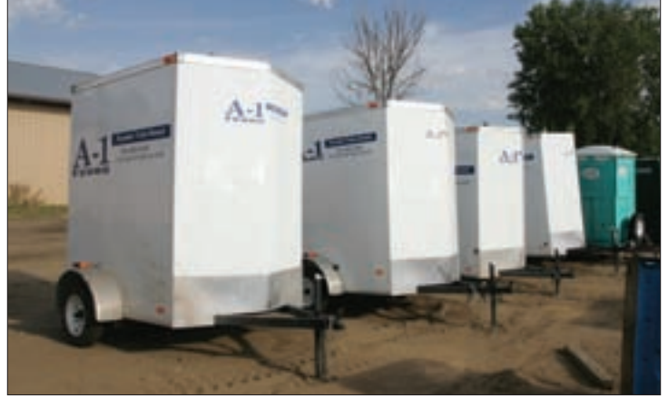
A-1 Evans builds these insulated single-unit restroom trailers, starting with the enclosed American Hauler trailer and adding a Satellite Industries toilet/holding tank and corner hand-wash sink.
