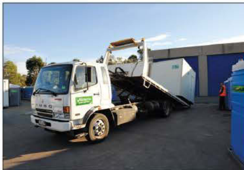
A cabover tilt-bed truck is used to deliver ablation blocks, skid-mounted steel-fabricated bathroom facilities commonly used in Australia.
