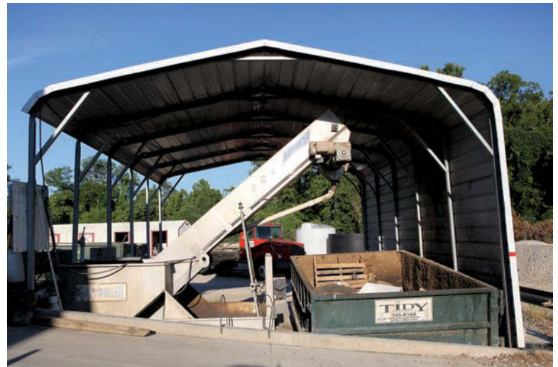
A Lely Maximizer dewatering unit is set up in the company yard, and sends solids into a container to be taken to a landfill. Wastewater is sent into the local sewer system.
