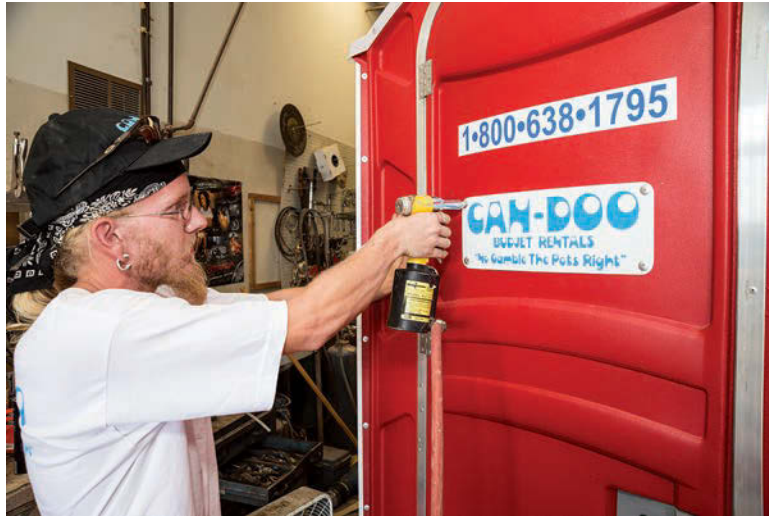
Above: Can-Doo employee Zack Bradshaw uses a rivet gun to affix the company's nameplate to a new PolyJohn PJN3 restroom.
