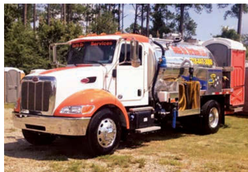
The new Gotta Go Services truck looks good and is built for driver convenience with suction and storage boxes on both sides and a twin restroom carrier on the back. (Photos courtesy of Wade and DeLaine Bernard)
