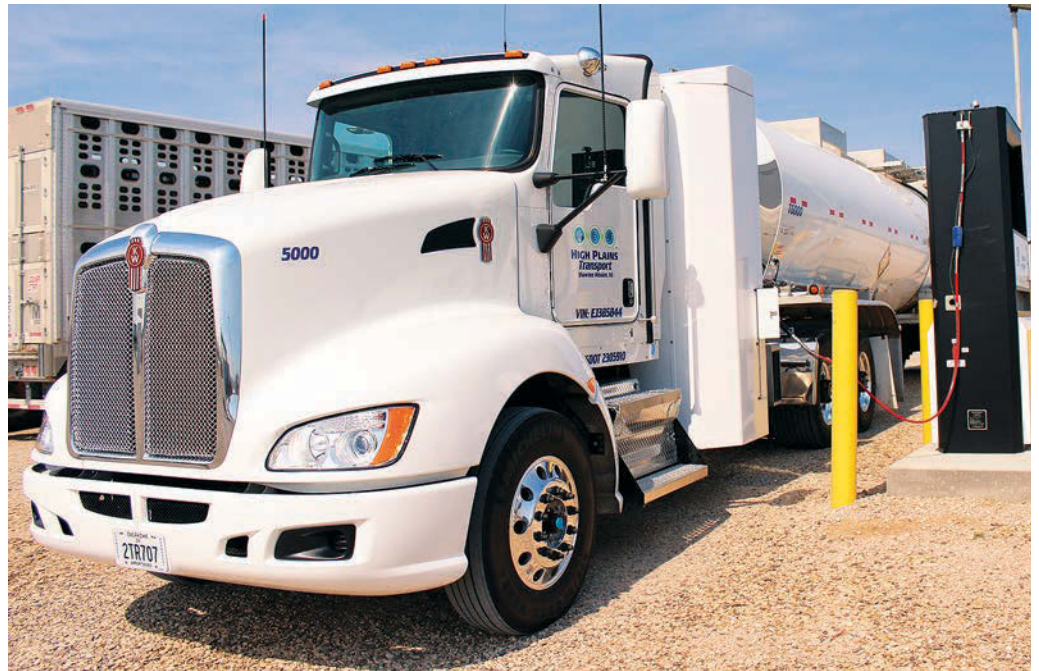
This High Plains Bioenergy rig is powered by a Kenworth T660 truck with Cummins Westport ISX12 G heavy-duty natural gas engine. (Photo courtesy of Kenworth)
