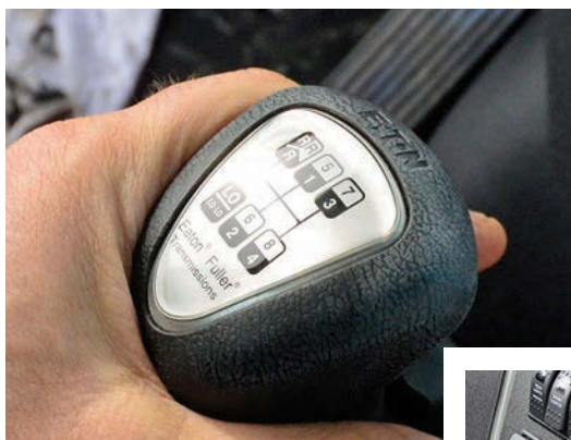
Above: Manual transmissions, such as this Eaton Fuller, place full control in the hands of the driver. (Photos by Ed Wodalski)
