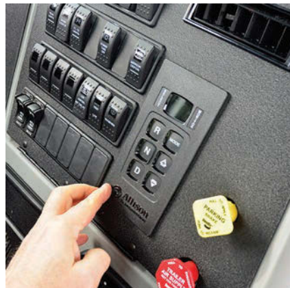
Right: The fully automatic Allison transmission relies on computer technology for optimum performance.
