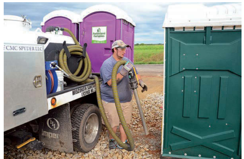
Below: Roberts is ready to empty another tank on his route that covers construction sites, businesses and other locations nearby in Wisconsin's Fox River Valley. His Ford service rig was built out by Imperial Industries with a Masport pump.
