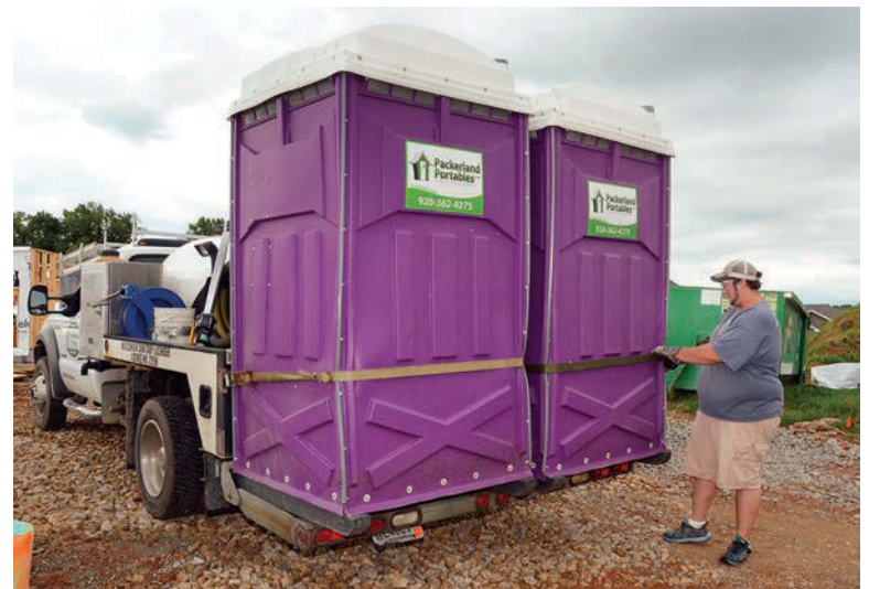
Before he heads off to another customer, Roberts checks the tie-downs on two PolyPortables restrooms that will be dropped off at a site later in the day.
