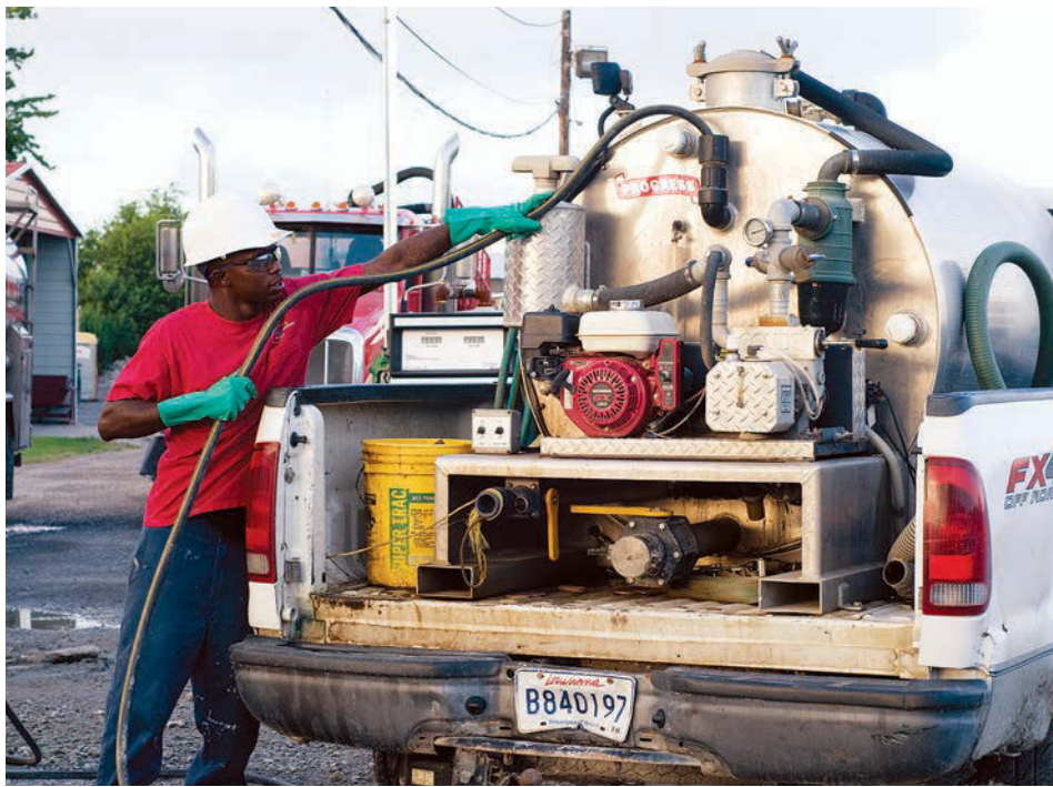
Left: Joe's Septic Contractors runs a variety of service rigs, from large to small. Here, technician Christian Berryhill uses a Progress VacTruck slide-in unit mounted onto the bed of a Ford F-150 four-wheel-drive pickup.
