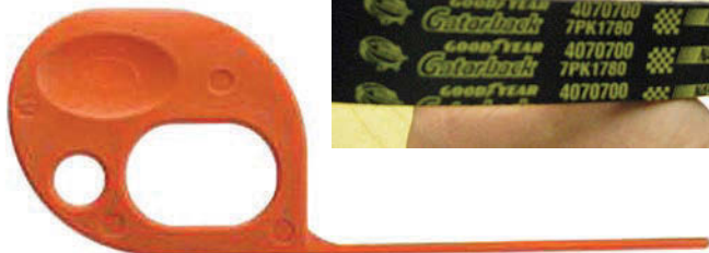
Below: Gates Belt Wear Gauge. (Photo courtesy Gates Corp.)
