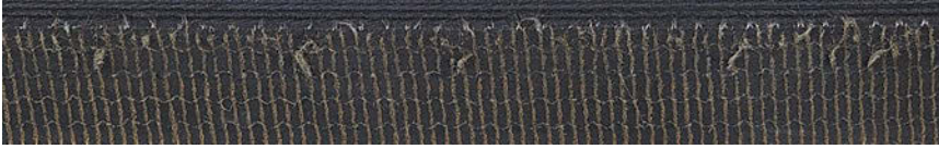
Worn backing means this belt has reached the end of its service life. (Photo courtesy Goodyear Engineered Products)
