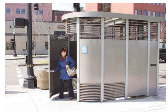
Right: The Portland Loo has a footprint of about 10 feet long and 6 feet wide with a rounded door on the front and an enclosed utility area in the back.
