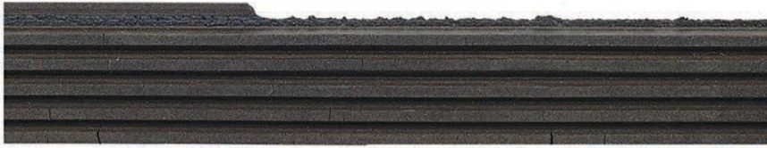
A missing rib indicates it's time for a new belt. (Photo courtesy Goodyear Engineered Products)
