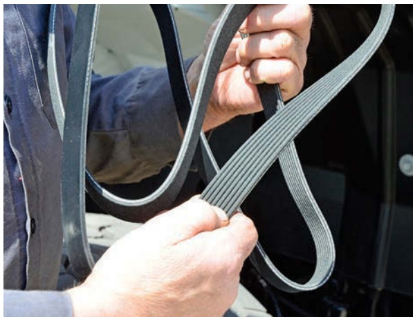
Above: Properly performing belts should be free of abrasion. (Photo by Ed Wodalski)
