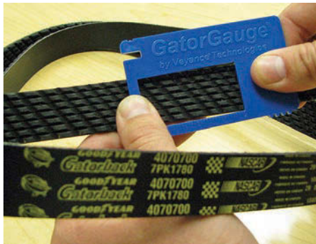
Below: Gates Belt Wear Gauge. (Photo courtesy Gates Corp.)
