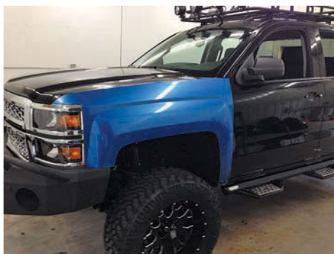
Above: Wraps are made from cast or calendered film and have a life span of up to seven years. Calendered film is best suited for flat applications, while cast easily negotiates the curves and contours of a front fender.
