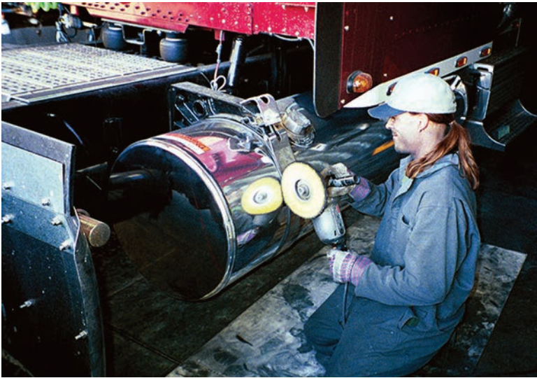
Above: An Air Vision technician cleans an aluminum tank using a high-speed grinder and the side of a canvas wheel.
