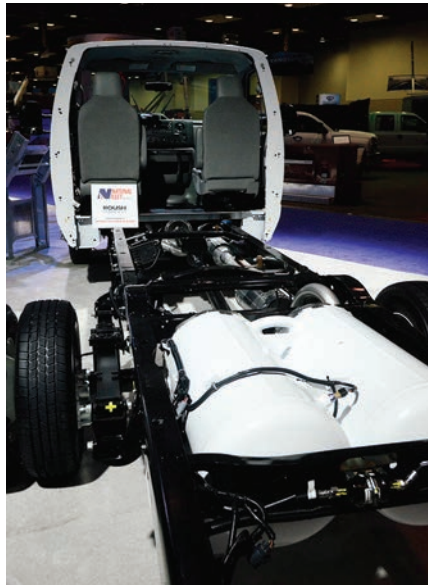
Left: A Ford chassis is outfitted with a Roush CleanTech dedicated CNG fuel package. (Photo by Ed Wodalski)
