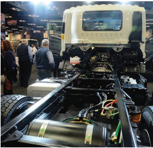
Isuzu Commercial Truck of America's cab-forward 2018 FTR chassis powered by a 5.2L turbocharged four-cylinder diesel engine. (Photo by Ed Wodalski)
