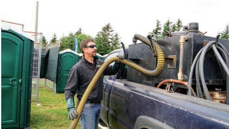
Stephen MacKinnon returns the hose to a 2003 Chevy service truck carrying a Crescent tank and Masport pump.
