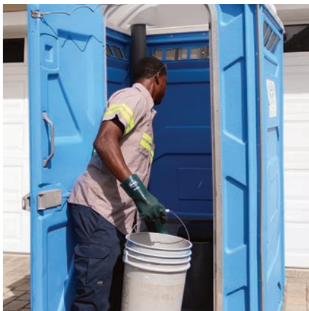
Kenneth Paul finishes up a unit service by recharging the holding tank with freshwater. The company uses deodorizing products from J&J Chemical and Walex Products.
