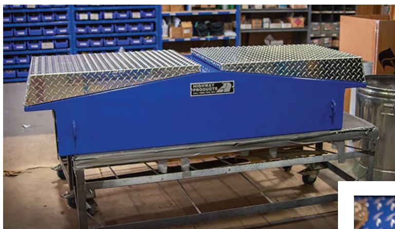
Above: A gull-wing hatch design offers convenient access from both sides of the truck. A single-lid crossover design allows bigger tools to be stowed in the box. (Photos courtesy of Highway Products)
