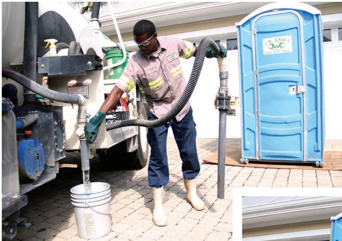
Left: Technician Kenneth Paul pulls the suction hose and pours a bucket of freshwater to prepare for a service job on a construction site.
