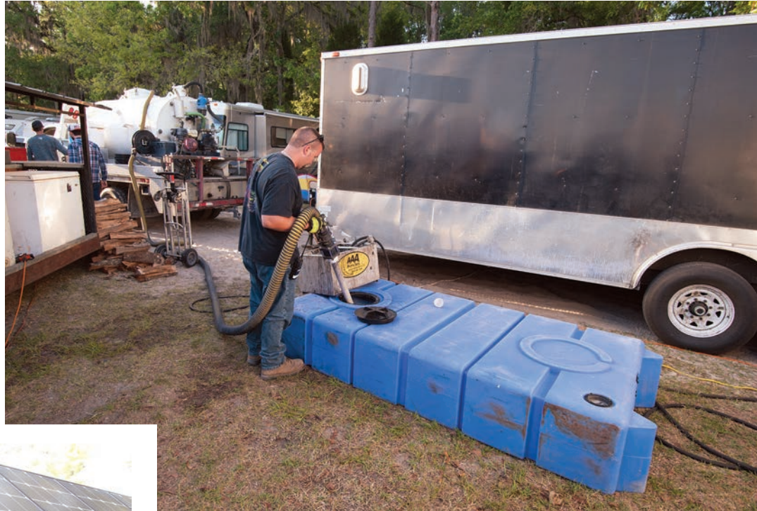
Above: Technician Dustin Fletcher pumps a Kentucky Tank holding tank at the festival. A strainer box built by AAA Porta Serve is seen on top of the tank. It is used to keep rags and kitchen debris out of the holding tank.
