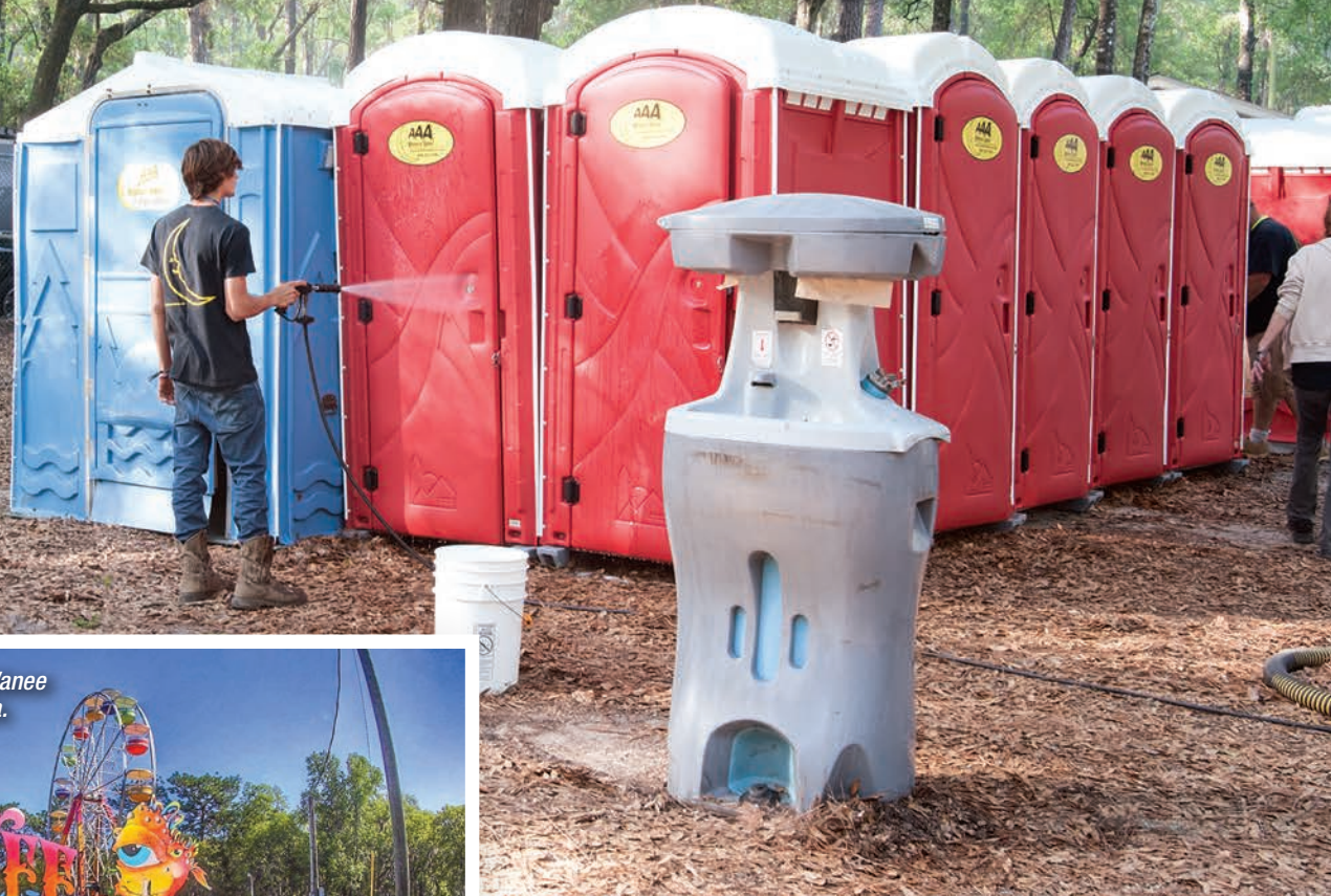
Technician Ryder Mock uses the Pathfinder Spray Cleaning System from Satellite Industries to wash restrooms. Restrooms are from Five Peaks, PolyPortables and Satellite Industries. A PolyJohn Enterprises sink is in the foreground. (Photos by Rob Herrera)
