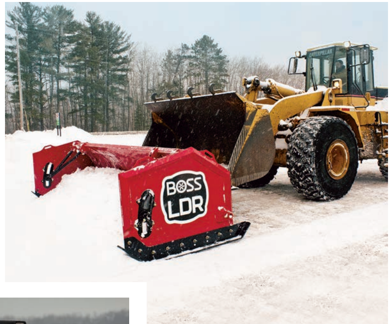
Above: A box plow attached to heavy equipment will clear parking lots quickly. (Photos courtesy of BOSS Snowplow)
