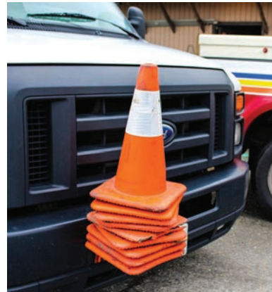
Left: A cone bracket is a smart way to carry bright orange safety cones on your work truck, ensuring your technicians are seen both while they are driving and when they are stopped on the roadside. (Photos courtesy of Northwest Cascade)
