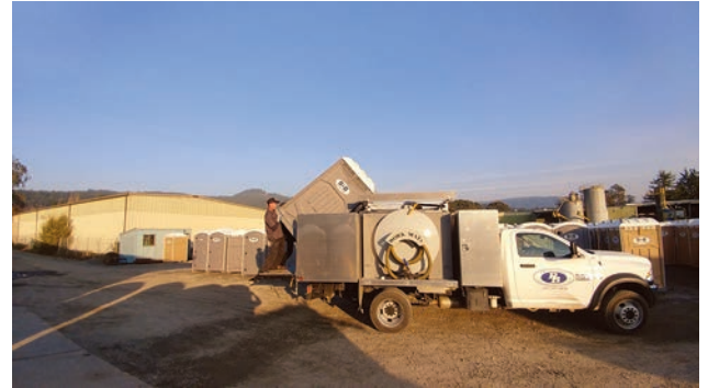
Below: Technician Robert Lawson loads a restroom for delivery on a service route. The truck is a Dodge 5500 built out by FMI Truck Sales & Service/WorkMate and using a Masport pump.
