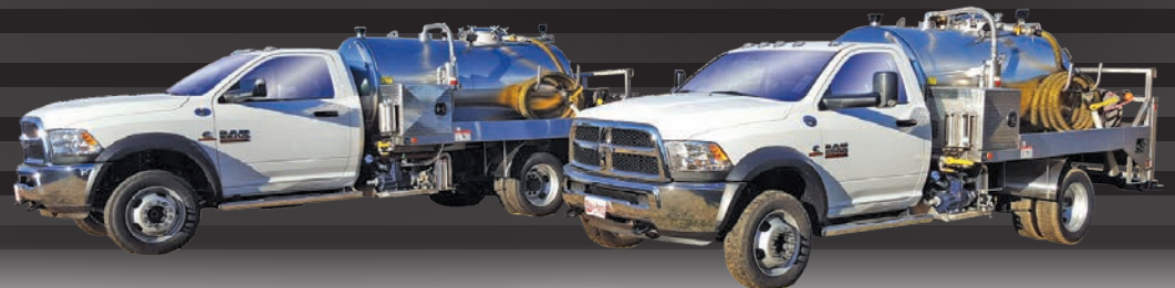
GH1100 800 waste/ 300 water mounted on a Dodge 5500
