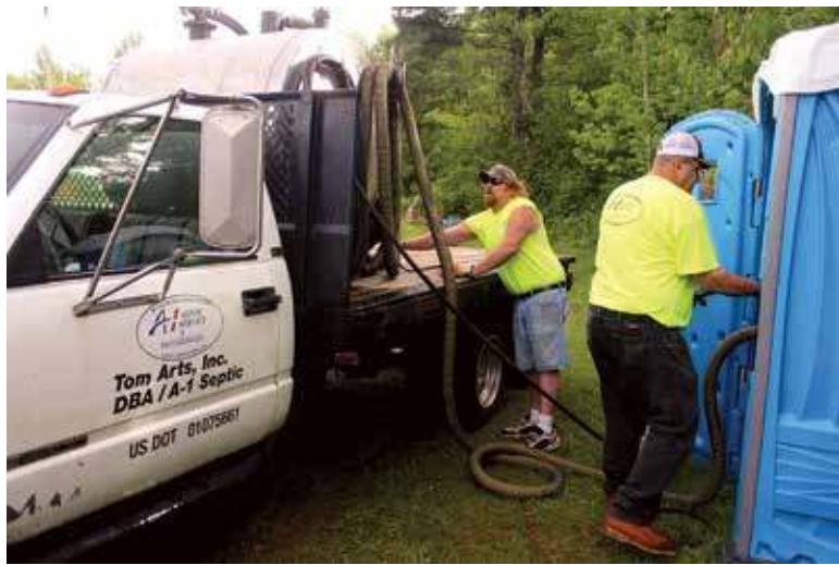
Clockwise from left: Greg Golden and Robert Lundberg service a restroom donated for the high school trap-shooting competition. The service truck is a GMC 3500 built out by Specialty B Sales with a 300-gallon waste and 100-gallon freshwater stainless steel tank and Jurop/Chandler pump; Technician Greg Golden delivers a pair of Five Peaks restrooms along the sporting clays shooting course using a trailer from Utility Trailer and a Polaris Sportsman 500 all-terrain vehicle; Competitors and volunteers walk the trap-shooting course at the Harshaw Sports Club. Restrooms were placed along the course to serve the participants.
