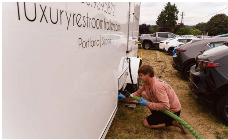
Robert Anderson prepares to empty the holding tank of a restroom trailer on location.
