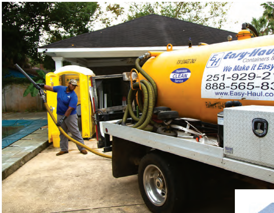
Above: Technician Joseph Mixon services a PolyJohn Enterprises restroom. His truck is a Ford F-550 built out by Lane's Vacuum Tank and carrying a Masport pump. Above, right: Technician Bennie Richardson logs service information on an iPad during his daily route. Right: At a wet and muddy construction site, Bennie Richardson washes the outside of a PolyJohn Enterprises restroom.
