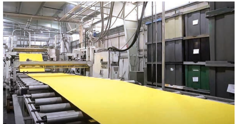
Above The extrusion line is where plastic pellets are made into sheeting.
