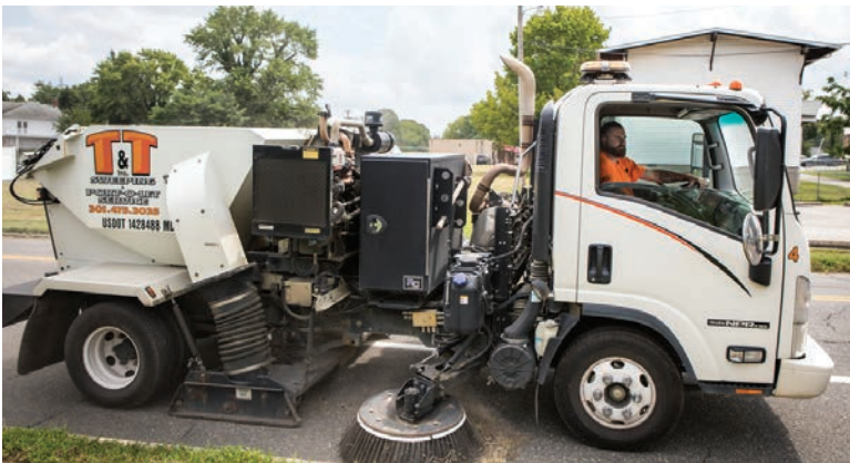
Above: Jeff Mundy operates a TYMCO street sweeper built on an Isuzu NRP truck. The company added portable restrooms to their established sweeping business.
