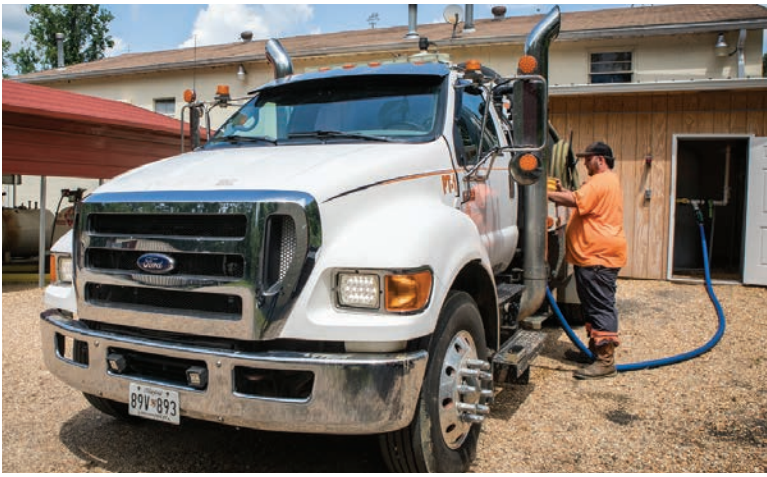
Above: Technician Austin Russell fills the freshwater tank of his service vehicle before starting a route. The truck is a Ford F-750 with a 1,100-gallon waste/400-gallon freshwater steel tank and Masport pump built by Abernethy Welding.
