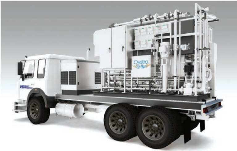
Above: This is a graphic artist's rendering of what a Wisconsin company's mobile septage treatment system looks like. The working prototype is 6 feet wide by 12 feet long by 8 feet tall and removes all pathogens from human wastewater.
