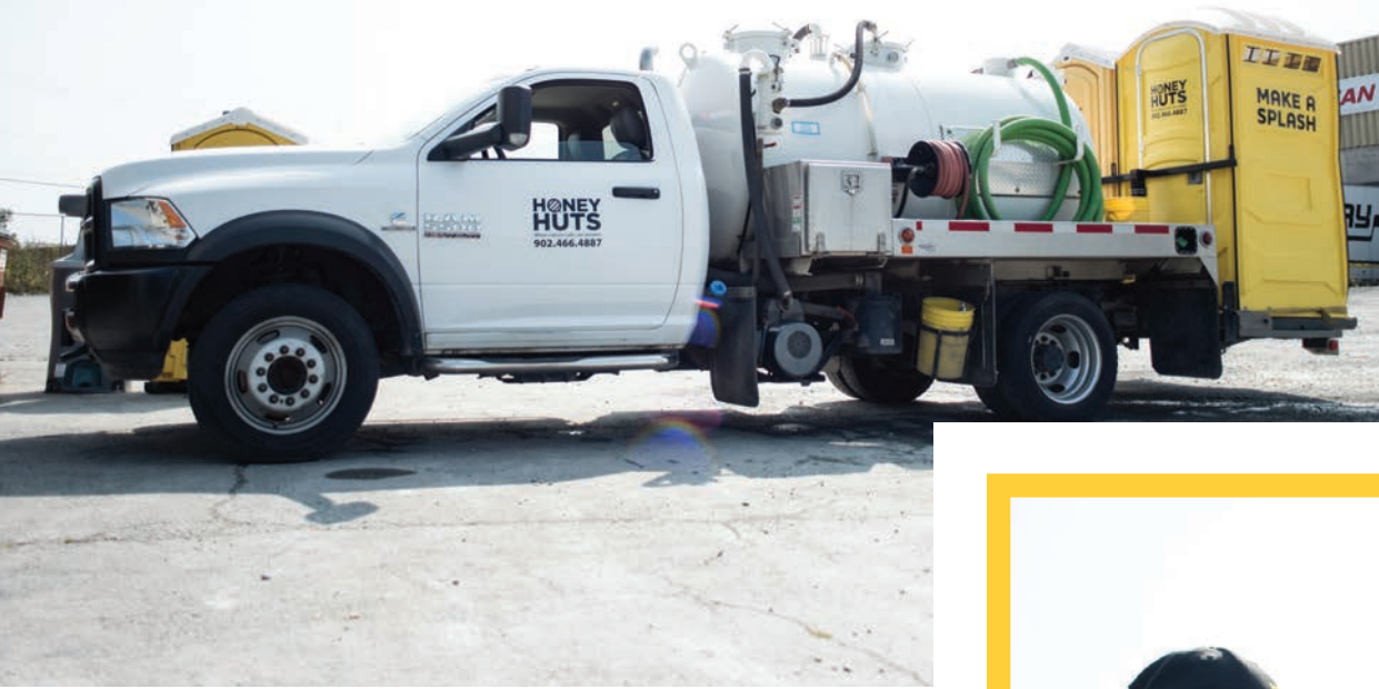
Left: A Dodge Ram 5500 from Vacutrix and carrying a Wallenstein pump is ready to deliver a pair of PolyJohn restrooms to a customer.
