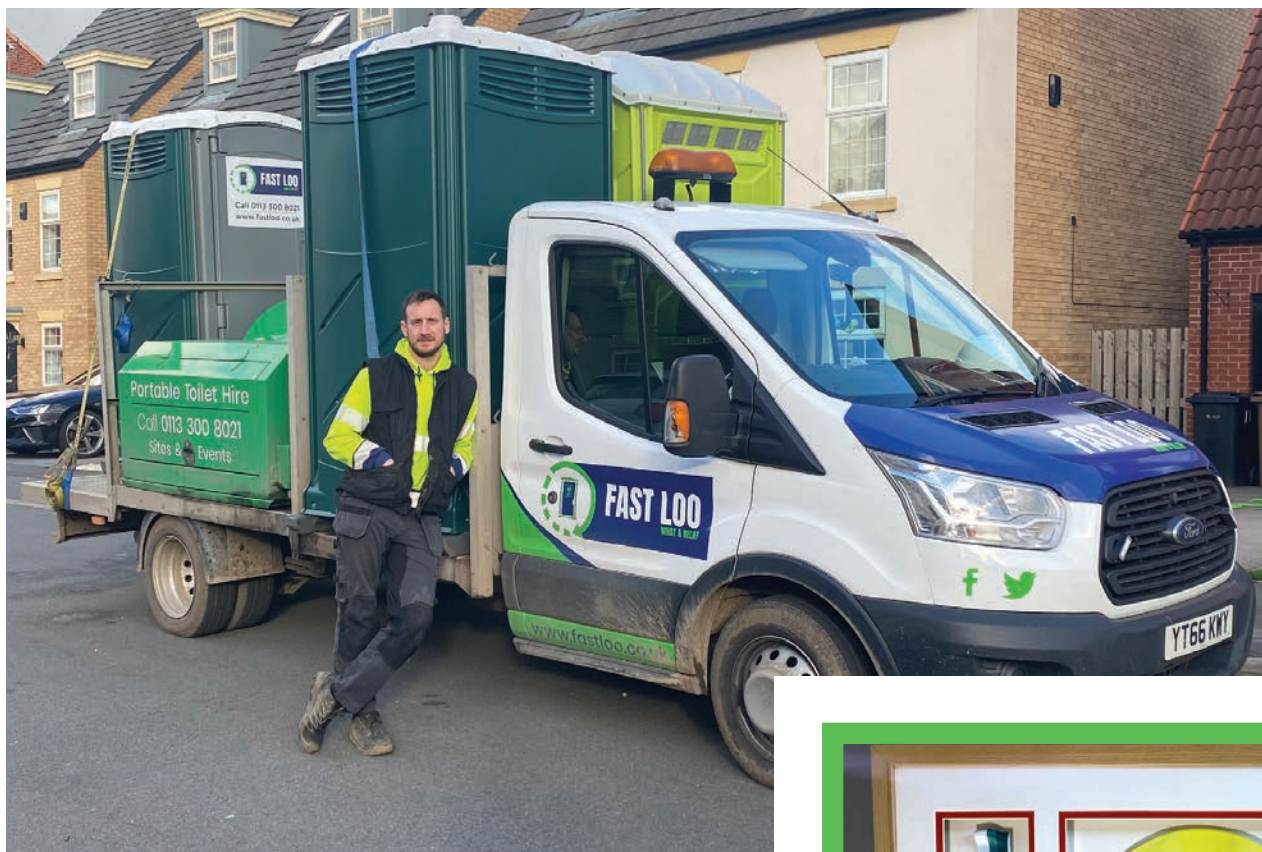
Left: Ibbetson is shown with Fast Loo's 2016 Ford Transit van converted to a flatbed by Rapide Tankers that carries four restrooms, a 180-gallon waste/100-gallon freshwater steel tank with a Honda GX240 pump, and a Honda GC160 power washer.
