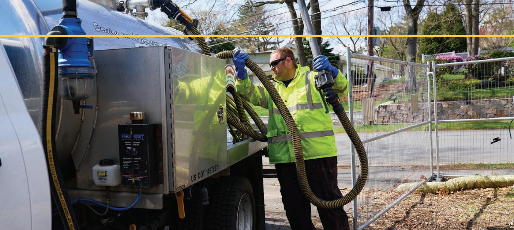
Above: On a service route, technician Kurt Sturtevant returns the vacuum hose to a Ram 5500 Service truck carrying a KeeVac tank and a Masport pump.
