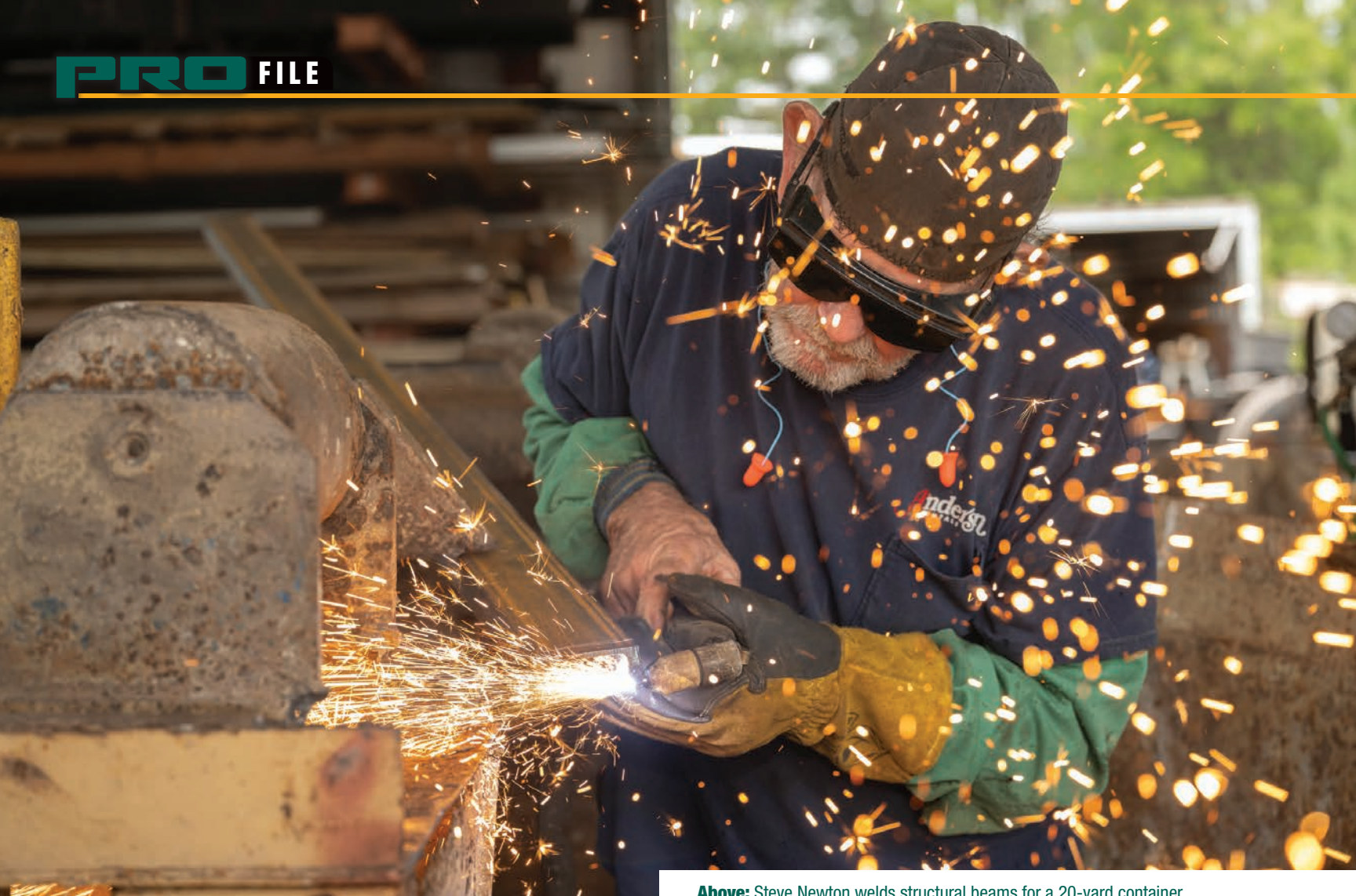
Above: Steve Newton welds structural beams for a 20-yard container at the Anderson Rentals facility in Mims, Florida.
