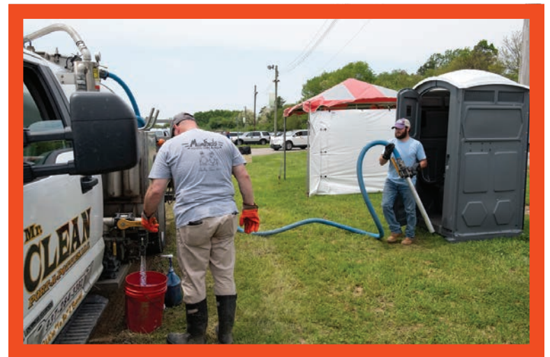
Right: Technicians Cameron Doggett, right, and Tony Rozmus service restrooms at the Clark County Fairgrounds, about 20 miles northeast of Dayton, Ohio. The truck was built out by Best Enterprises and carries a Masport pump.
