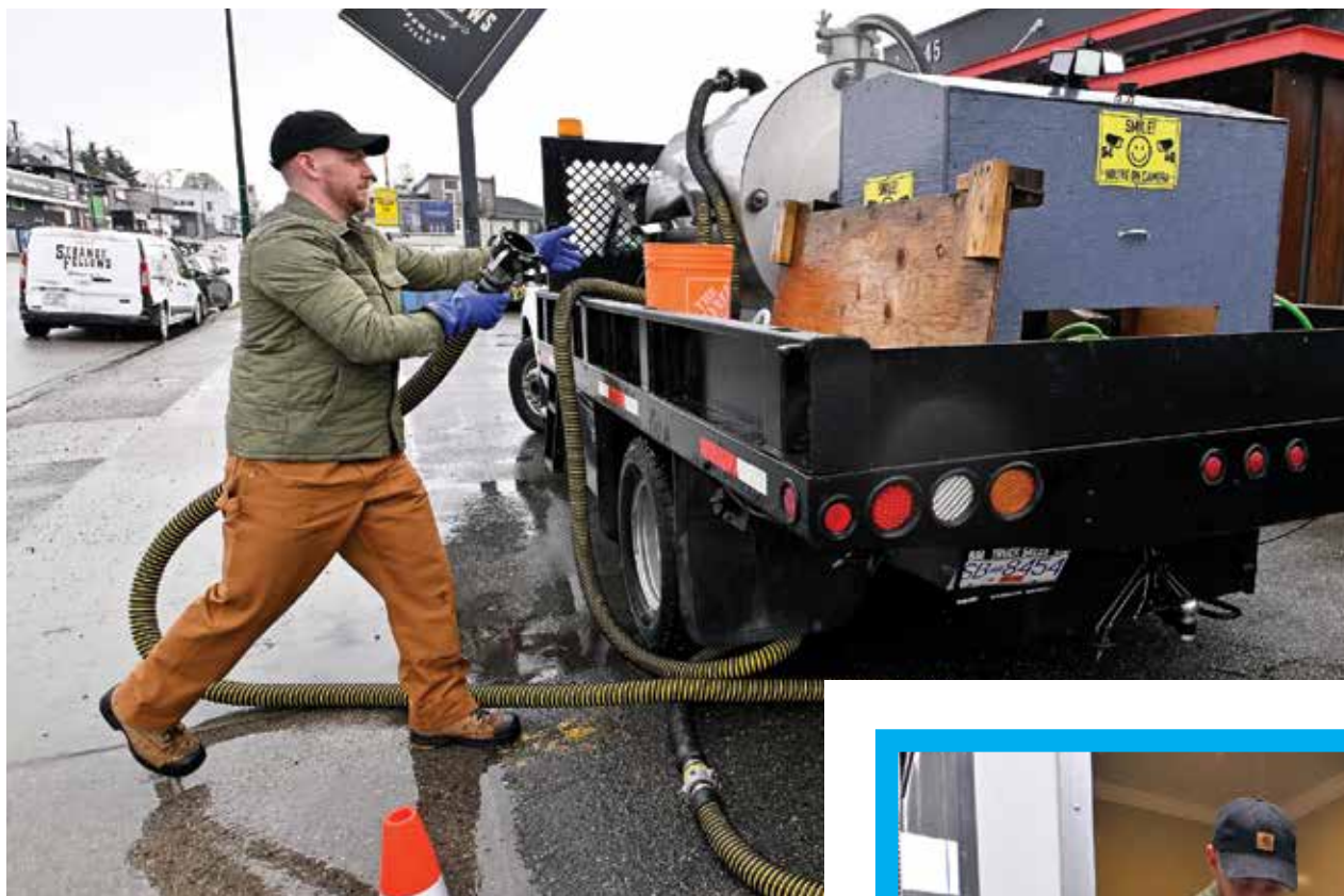
Left: Bluejay Rentals outfitted a Ford F-350 flatbed with a vacuum tank from ITI and using a Masport pump. Bradbury is shown servicing his trailer at a local brewery.
