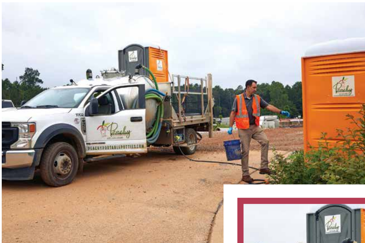
Left: Elliott carries water to recharge a serviced Armal restroom at a construction site. His truck is a Ford F-550 built out by Robinson Vacuum Tanks with a Portalotgix tank and Masport pump.
